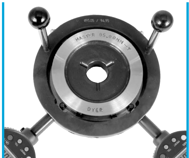
283 Special OD gage position on cylinder master.
