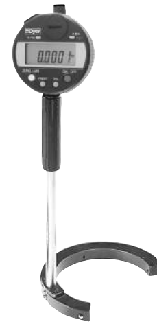
Measure precision bore with part fixture obstruction, on the machine
