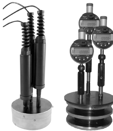
3 Ø's, Taper, out-of-round, TIR
