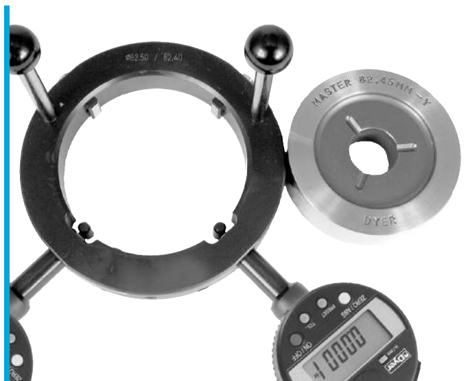
283 Special OD gage to measure splined part.
