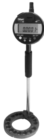
282 Series individual model to measure ID over hub, bore is deep into part
