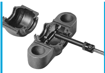
Gage open to measure larger internal bore
