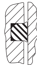
Corner build-up can result in excessive pressure that can lead to O-ring failure
