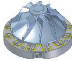
5-axis turbine blade machining
