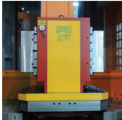
2-sided EPM on palletized system
