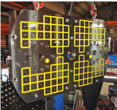
Load and install PIM magnet with bolts
