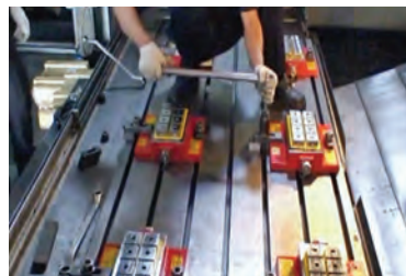
Lock them in position using bolts provided
